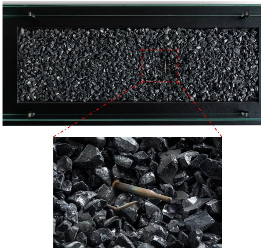
Fig. 2 – FIKA top view and ignition elements detail
