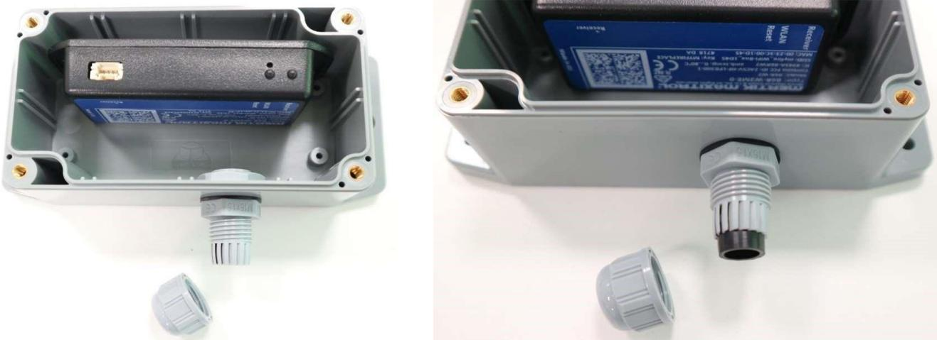
Place Wi-Fi Box cable through the nut (first) and sealed cable bushing into the protective box. Make sure that the rubber gasket stays on place
