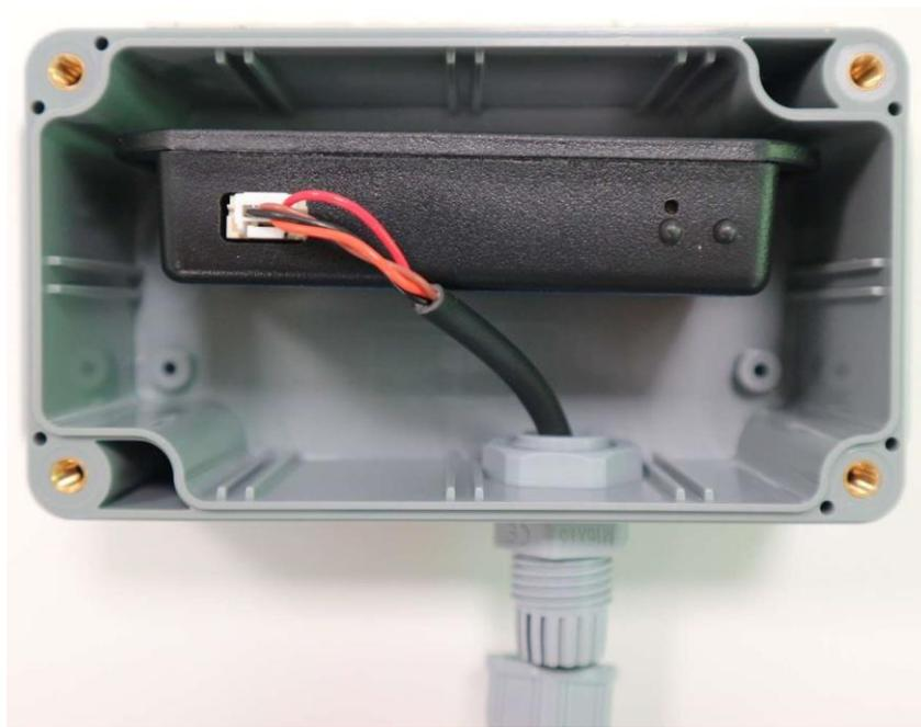
Screw the nut to seal the connection
