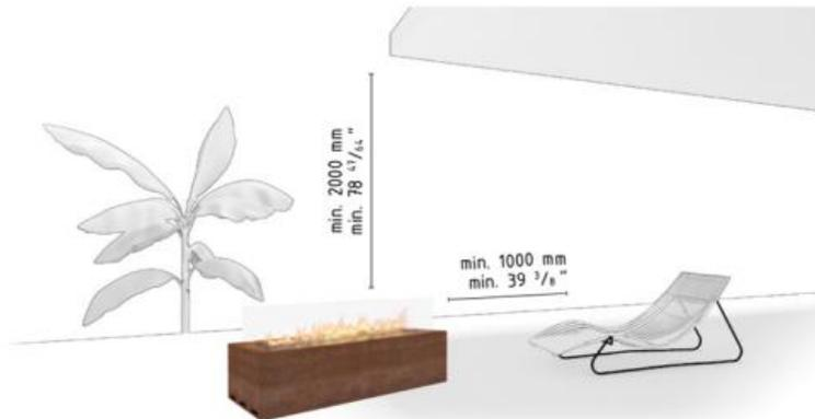
*Fig. 1: Minimum distance to flammable materials*
